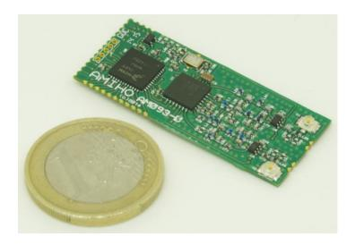
The AM093 Wireless Meter-bus (W-MBus) 169/868MHz modem uses the Freescale KL26 Kinetis ARM Cortex M0 microcontroller and a Semtech SX1276 Radio Transceiver to form a compact dual band 100mW module.
