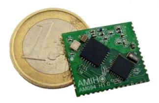
The AM094 LoRa / LoRaWAN / Wireless Meter-bus (WM-Bus) 868MHz modem uses the Freescale KL16 Microcontroller and Semtech SX1272 LoRa / Narrow band transceiver to form a compact 25mW module.
